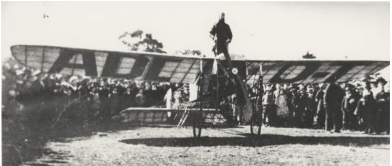
nla.pic-vn3723553; First flight from Melbourne to Sydney showing pilot Maurice Guillaux standing on a Bleriot monoplane with a 50 horsepower Gnome engine, Wangaratta, July 1914 (E.A Crome collection)
