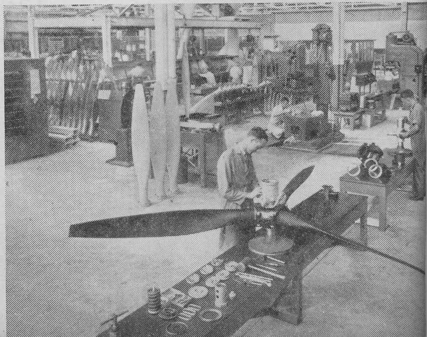
Final assembly section in the de Havilland Propeller Division, which is now producing propellers for the Mustangs, Lincolns and Mosquitos.
