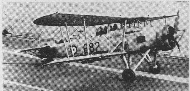
Fairey Swordfish landed-on HMS Courageous . Note extended landing arrester cable attached to hook. Date 1938.
