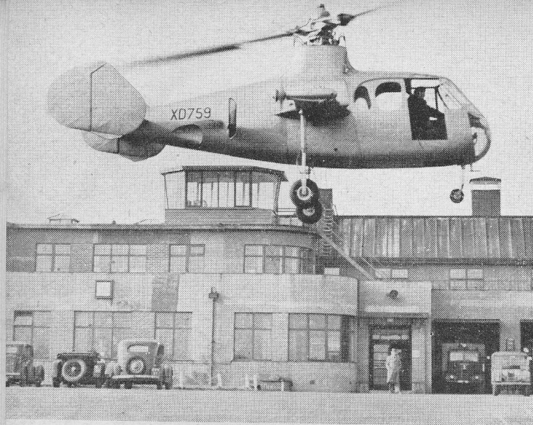
Fairey's have engaged in extensive helicopter research. This is the Jet Gyrodyne for tip-jet propulsion experimentation.
