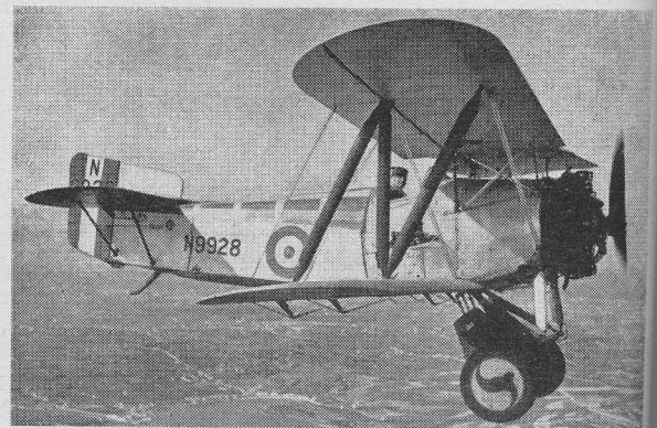
LEFT: The Atalanta flying boat of 1928 fitted with four Rolls Royce 650 HP Condor III engines paired in tandem. A.U.W. was 30,500 lb, span 139 ft, length 66 ft, service ceiling 14,100 ft. RIGHT: The Flycatcher, an outstanding deck-operating fighter of the 1920s. Fuselage "broken-back" gave big wing angle when tail-down with short undercarriage.
