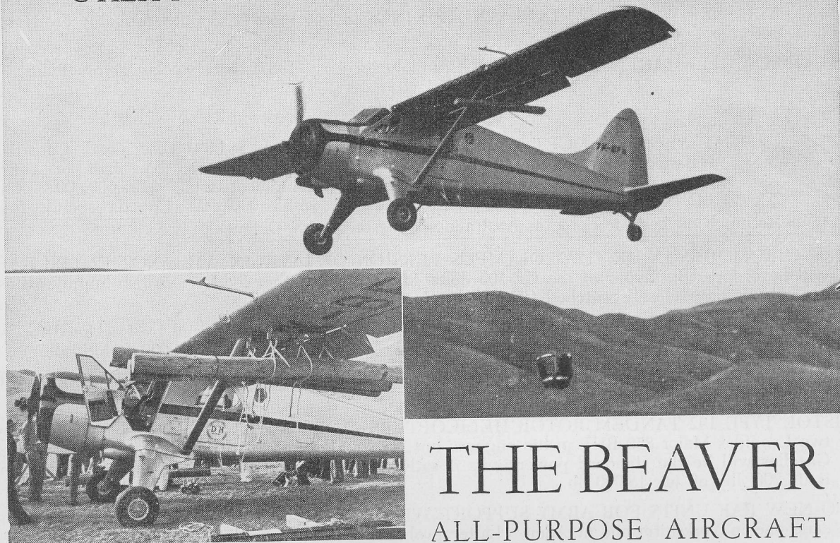
THE BEAVER SHOWING WING ATTACHMENTS Posts being carried on supply-dropping racks of the De Havilland Beaver. The posts are 11 ft. long and 8 in. in diameter and weigh approximately 130 lb. each.
