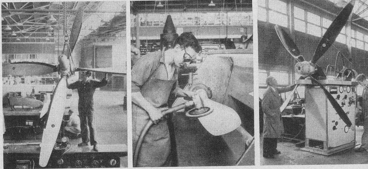
The de Havilland Propeller Division at Alexandria is well equipped to service commercial and military equipment. LEFT: Bristol Freighter propeller built by de Havilland Propellers (England) is lowered onto a test rig. DH overhauls and rebuilds Hamilton-type propellers in Australia, including those used by major airlines. On bench at rear is Hamilton-type propeller built by de Havilland Australia. CENTRE: Blade finisher polishes and buffs a reconditioned propeller blade preparatory to anodising. RIGHT: Alexandria is frequently called upon to service non-DH equipment. Here a rear Rotol propeller from a Gannet contra-rotating assembly is subjected to a functional test on a Rotol test rig.
