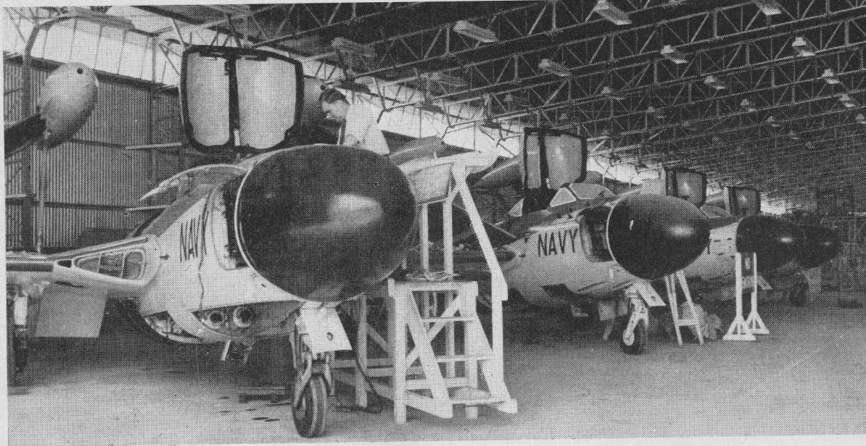
Part of Sea Venom line in new service hangar. Aircraft are at Bankstown for ejection seat installation and overhaul.
