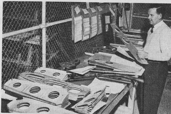
Wing main ribs awaiting check in the View Room.
