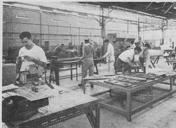
LEFT: Another general view of the aircraft shop with the tool room in background. In foreground, chief inspector Doug Wilson discusses with the shop foreman details of rib form tools. Press brake in background is testing "T" section form tools. RIGHT: A wing assembly jig in construction. Immediately behind it can be seen the spar and nose rib assembly jig.
