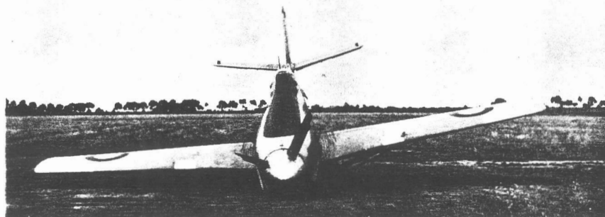
(Above) The CA-15 after it crash-landed at RAAF Point Cook on 10 December 1946, after a failure in a pressure gauge had allowed all the hydraulic fluid to drain out of both the main and the emergency hydraulic systems. (Below) The CA-15's cockpit showing the flying instrument panel. The throttle, propeller controls, fuel levers, and u/c, flap and trim selectors were grouped on the left and electrical and hydraulic controls on the right side of the cockpit.
