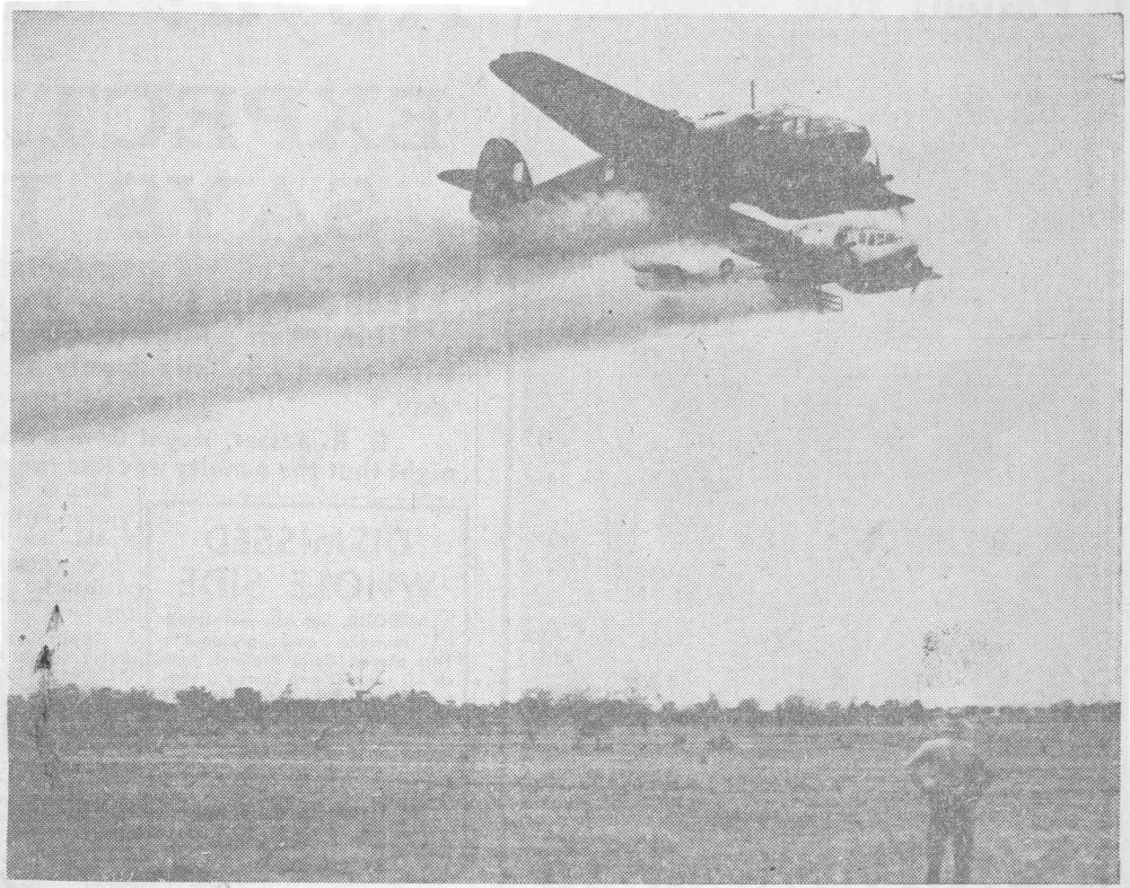
R.A.A.F. BOMBERS spraying gammexane at a cost of £1 a second in the air war against the Mallee (Victoria) grasshopper plague.
