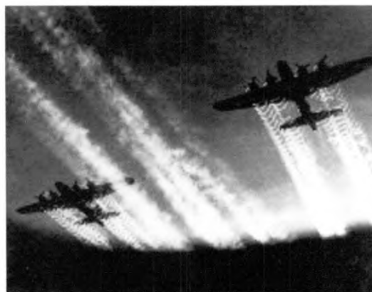
An interesting photograph of aerofoil tip vortices, you can see the propeller pitch - a B17 Flying Fortress?
