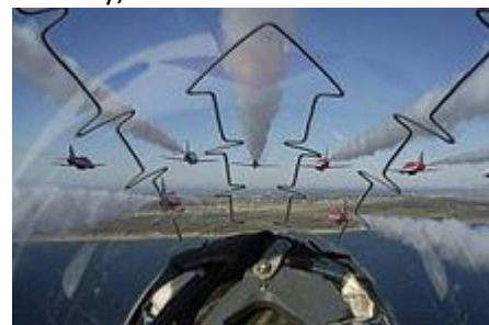
A cockpit view from a BAE Hawk showing the explosive cord in the canopy
