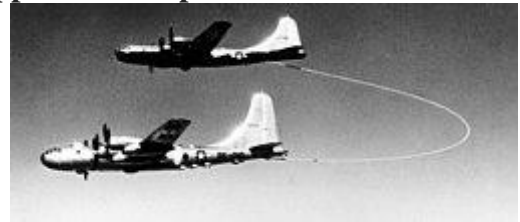
The US Airforce Boeing B-50 Superfortress, Lucky Lady II being refuelled by Grappled-line looped-hose during the first non-stop circumnavigation of the world by air (1949)
